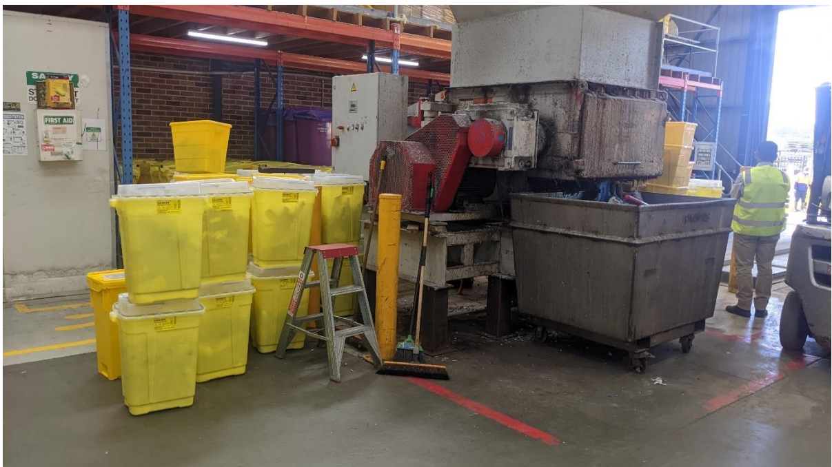
Photo 2 – The shredder used to shred clinical waste after treatment in the autoclave.
